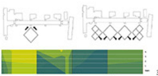
facade daylight study for slab concept 55% in shadow
